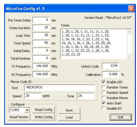
Morse code ID. It then will stop transmitting, and repeats every 30 seconds. The only setting users must change is the Morse Code ID text to be their assigned amateur radio callsign. After setting the desired options, select the configuration cable COM port, connect the cable to the 2.5mm jack on the MF2, being sure to push the plug all the way in, switch on the power and press Read Version, then Write Config to apply the settings.
